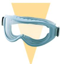
*Direct-vented goggles* allow surrounding air directly into the goggles. They are used primarily to protect against projectiles. **They do not provide adequate protection against splashes or vapors.**
