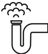
The negative air pressure ventilation in a laboratory is more likely to pull up odors from a drain than an office (which has positive pressure ventilation). Dry traps could occur in “cup sinks” (small sinks in the middle of lab benches), floor drains, and sinks covered by equipment or no longer used. Prevent or eliminate dry trap odors by running water in all sinks with a ½-gallon of water once a month.
